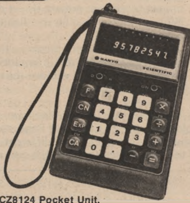
CZ8124 Pocket Unit. A complete 8 digit "economy" scientific calculator with 2 digit exponent. In addition to its basic functions, it has a fully addressable memory, exponents, log, pi, 1/x, \, ex, sin, cos, tan, sin -1 , cos -1 , tan -1 , radians and degrees. AC or DC power. $80.50 without AC adaptor.
